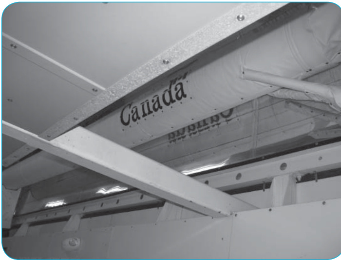
FIGURE 5 Canadarm in its folded configuration, stowed aboard the Space Shuttle Explorer. The robotic arm was used for servicing items in space. (Photo courtesy of P.E. Weiss.)
