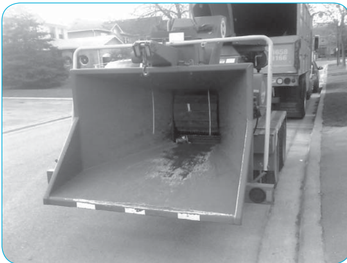
FIGURE 2 Hopefully no one would try to retrieve this coffee cup from the inlet of the wood chipper! It is difficult to guard a wood chipper to prevent humans from being killed, since large tree branches must be fed into the blades. This unit is equipped with two “last chance” safety straps in the chute. If these are pulled, the chipper feed reverses immediately.
