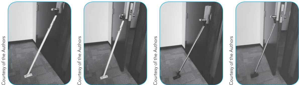
FIGURE 1 An example of a “workaround.” The variable length security bar was designed to wedge a door closed but to contract in length a fixed amount so that the door could be opened a bit, while still preventing an intruder from entering. The needed telescoping action is created using telescoping tubes (seen on the left), and this design was protected by US Patent 5988710. The design shown on the right contracts without telescoping tubes using a flap at the foot end, and hence “works around” the patent to achieve the same functionality without infringing.
